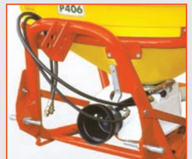
Oil hydraulic drive.
