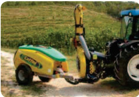
The trailed sprayer thanks to its articulated system (the head of pulverization complete pump, turbine, diffusers are mounted on the tractor hitch and the tank is trailed) allows unthinkable steering angles compared with other atomizers. Furthermore, the PTO shaft works straight.
